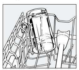
There are angled holders in the corners of the upper basket. These are made to support narrow glasses in the best position for a thorough cleaning.
